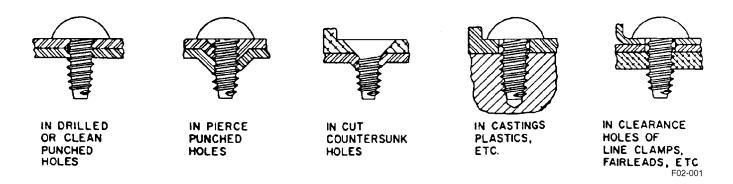
Figure 2-1. Using Sheet Metal Screws
