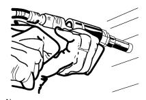
Above: Automatic Driver assembles HI-LOK Collar on Pins. Interference fit holes can be prepared and HI-LOK Pins inserted by Drivmatic Riveter method.
